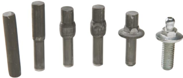
**Cold forming progression:** Above, parts first start as a raw blank and then are progressively formed with dies to shape and trim parts.
